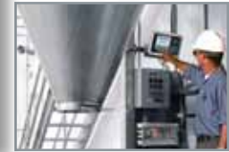
A 32-channel display capability allows viewing of weight on an individual scale and a combination of totalized scales.
