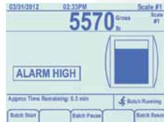
Bar graphs and visual cues inform users when a batch or fill is in process and when it's approaching target weights.
