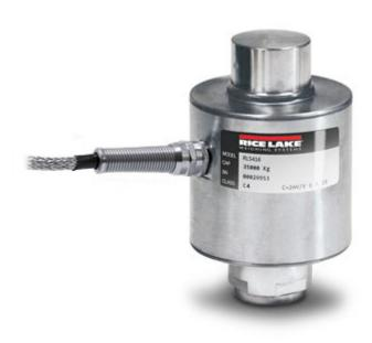
Canister load cells for CE-M approved weighbridges, tanks, silos, etc. Manufactured in STAINLESS STEEL, IP69K protection degree, 4000 divisions.
