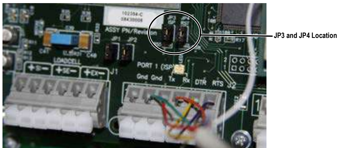
Figure 8-4. Jumpers Installed on JP3 and JP4
