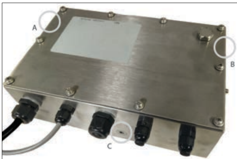
Figure 2-8. Paper Sealing Method
