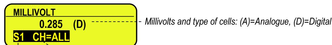
*Checked channel / digital load cell.*
