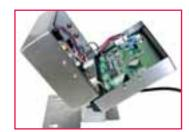
Internal Hinge Mechanism
