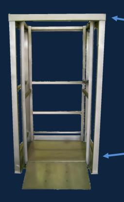
Designed similar to the PB3000 system where a weigh frame is separate from the sub frame via ball races. This ensures any side shocks are taken up through he frame not the load cell
