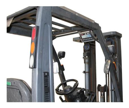
Weigh System Designed and Manufactured in Australia by Associated Scale Services
