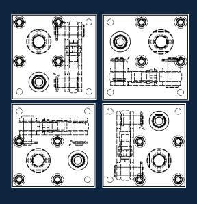
Suggested orientation for optimum weighing and stability. 10t- 30t
